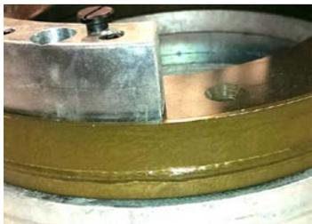
Position drill bushing over broken bolt and
