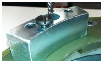
Remove 5/32" bushing, using reverse
