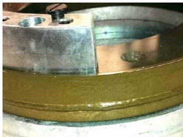
Position drill bushing over broken bolt and attach to light base using provided flat head bolts.
