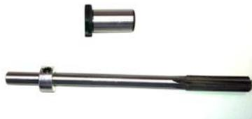
If you have spacer rings and/or flange ring, insert 1/2" bushing and use reamer to enlarge through holes in spacer rings and/or flange ring-ONLY. Use depth gauge to avoid reaming top flange hole- **DO NOT REAM OUT** top flange of base and/or top flange of extension or top section.
