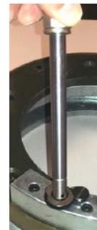
Insert 1/2" bushing into bushing block. Liberally apply tapping fluid to insert and drilled hole. Attach wrench on the cap screw and turn in the threaded insert until the installation sleeve bottoms out on top of flange. Insert should now be installed flush to top of flange.
