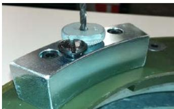
Use 5/32" drill to core out center of bolt
