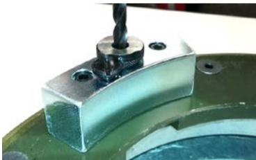
Use 15/32" drill bit, drill hole in top flange. Drill through spacer rings if applicable. If you do not have any spacer rings and/or flange rings, go to step #6.
