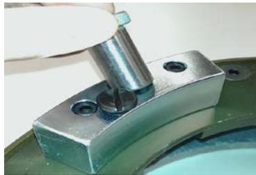
Insert 15/32" bushing into bushing block. Apply liberal amount of tapping fluid.
