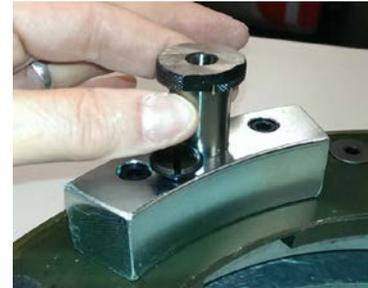
Insert 5/16" bushing into bushing block.
