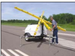
3. Tilt the light to the upright position.
