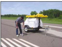
1. Level as necessary using 3 leveling jacks.
