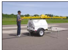
2. Extend the 4 light assembly arms.
