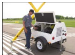
4. Start the generator and activate the lights.
